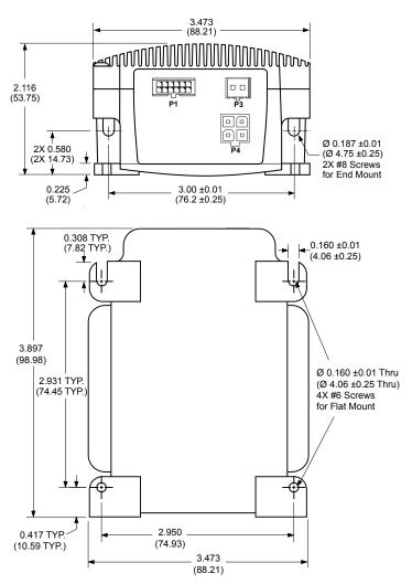
Figure 1.2.1: MForce PowerDrive Mechanical Specifications
